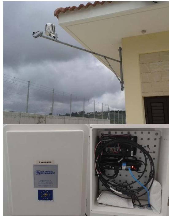
Figure 1. SmartPV weather stations that assist in forecasting PV generation.
